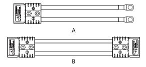
Anderson connector is used on the DC input side of wall mounted battery series. The specific connections are as follows:
